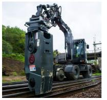
**Requirements of Excavator Operating pressure Operating pressure Back pressure** Recommended oil flow **Recommended oil flow** open/close rotate open/close rotate max. 35 MPa (350 bar) / max. 14 MPa (140 bar) / 0,5 MPa (5 bar) / 150 - max. 250 l/min / 18 - max. 25 l/min / 5040 psi 2016 psi 720 psi 39.6 - max. 66 GPM 4.8 - max. 6.6 GPM
