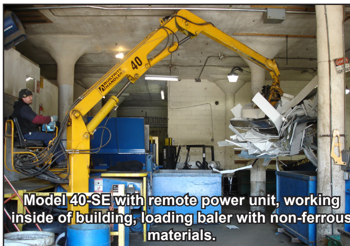
Model 40-SE with 18' Material Handling Boom. Operator's platform is attached to tower. Power Unit is remote.
