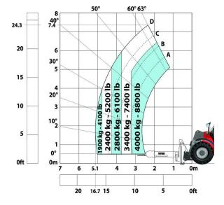
Machine on tyres with tyre handler TH 49 (Imperial)
