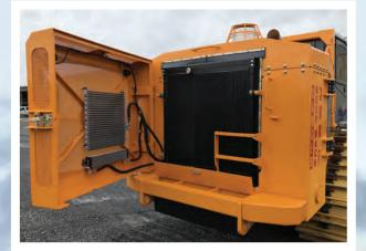
HIGH EFFICIENCY COOLING PACKAGE WITH COARSE FINS FOR EASY CLEANING
