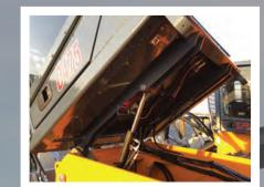
PUSH BUTTON CAB TILT FOR EASY ACCESS TO COMPONENTS & HYDRAULIC OIL FILLING PUMP
