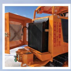
HIGH EFFICIENCY COOLING PACKAGE WITH COARSE FINS FOR EASY CLEANING
