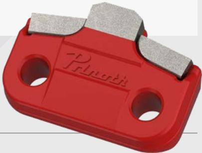
Triple-carbide tool with main cutting tip in the center, side tips set diagonally to reduce power requirement, for wear-intensive and sandy applications.
